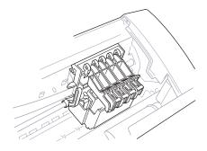
**3** Open the ink cartridge cover by pinching the clip as shown in the illustration.
